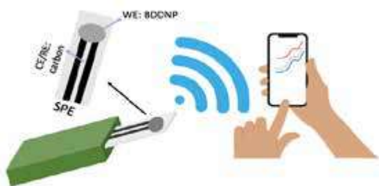
Figure 1. Sensor device using screen printed diamond electrode
