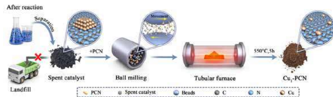
Figure 1. Solid-phase upcycling process of ultrahigh loading SACs
